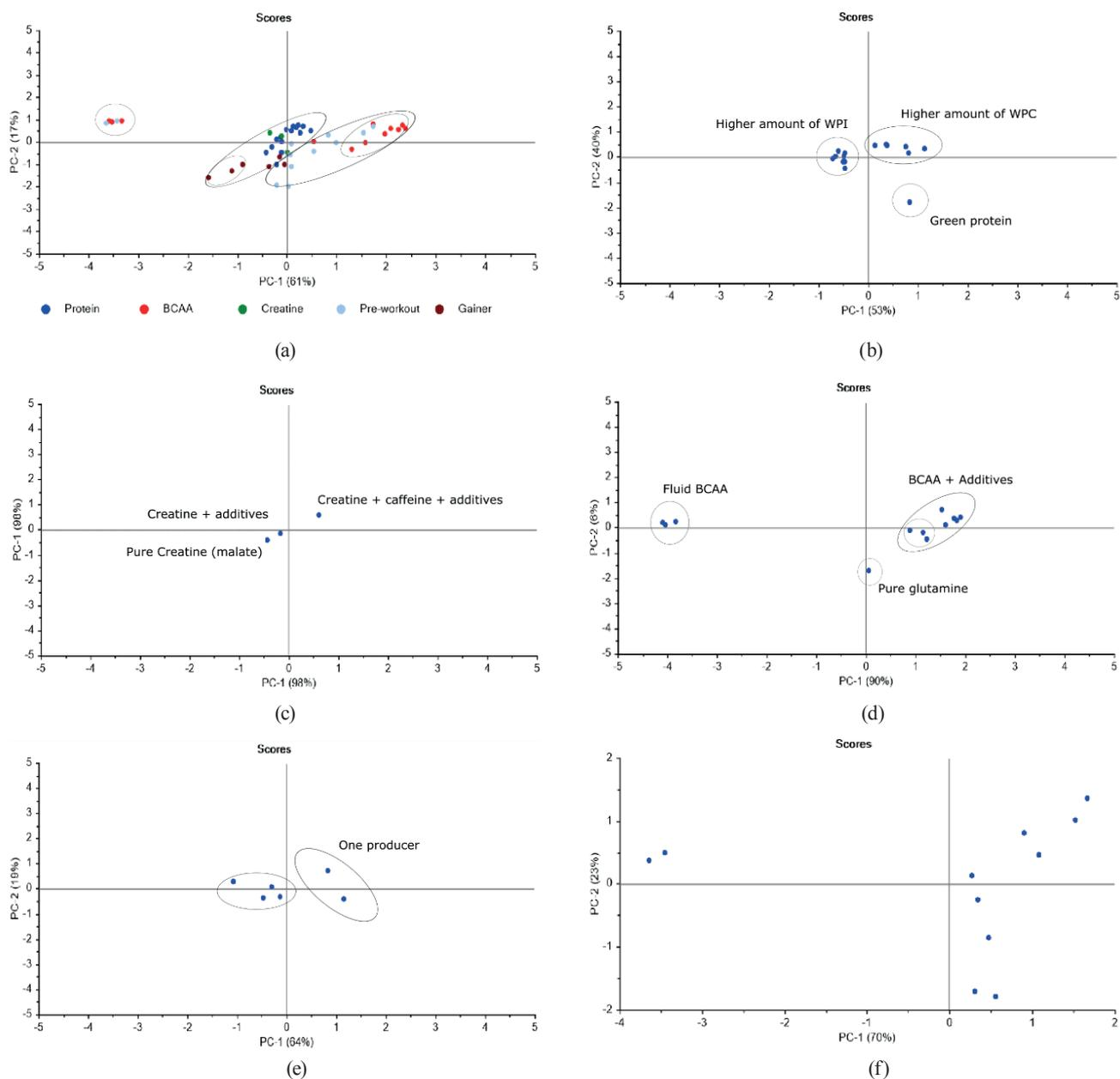
**Figure 2** PCA results for medium infrared spectra of sports supplements. Scores plot for two significant principal components: PC1 vs PC2. (a) all samples and full spectra at 4000–600  $\text{cm}^{-1}$ ; (b) proteins; (c) creatines; (d) BCAA; (e) gainers; (f) pre-workouts [22]
